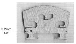
Insert the transducer into the hole that you have drilled. It is important to make sure that the line on the transducer tip is horizontal as you insert it into the bridge. In order to ensure that the active part of the transducer is completely inside the bridge, you should be sure to insert the transducer to the point where its tip is in contact with the flat end of the hole. The transducer is designed to be a snug fit in the hole.
